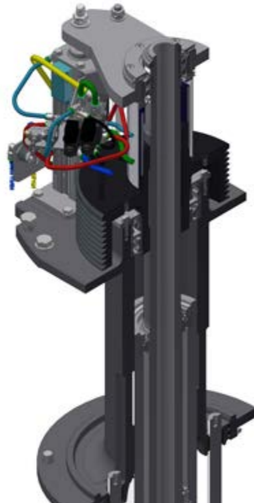
Oransal valf detayı – enkoderli silindir Detail of the proportional valve – cylinder with encoder
