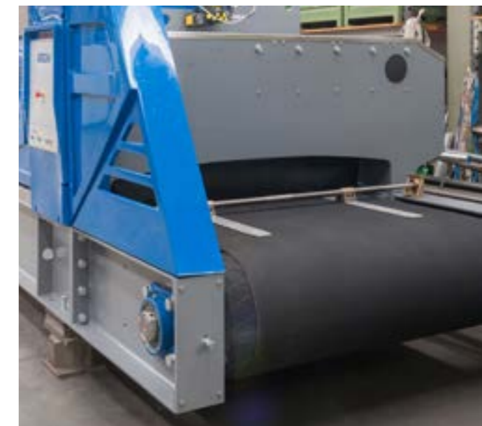
Detalle de la guía de azulejos / placas Detail of the tile/slab centring rails' valve
